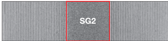
Under microscope at 100x magnification The core material is SG2 and is covered by 80 layers on each side.
